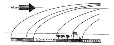
Internal boundary layers are significantly developed disturbance layers in the near-surface layer, which are generated by horizontal advection over discontinuities of the surface properties (roughness, thermal properties, ...)
