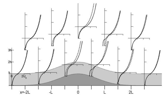
Finnigan and Belcher (2004) Belcher et al. (2007) This tendency for the wind to blow toward the crest of the hill on both the upwind and lee slopes within the canopy leads to a convergence of air at the crest of the hill. There is then an ejection of air out of the top of the canopy at the crest of the hill.
