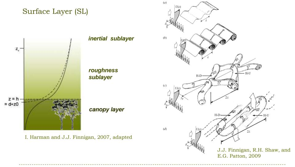
canopy flow fundamentally differs from flow in the logarithmic layer: scaling of turbulence moments does not depend on distance from the ground but is dependent length and velocity scales related to canopy geometry
