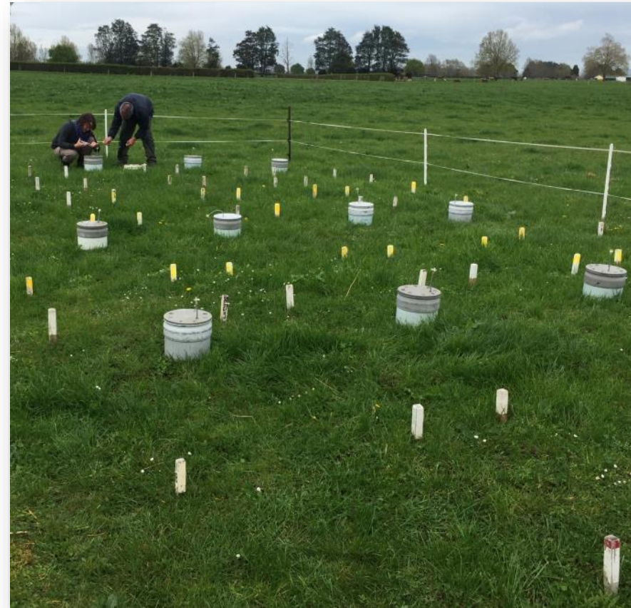
Small plot N 2 O trial at Troughton Farm showing manual flux chambers
