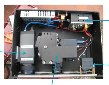
Support electronics & Arduino processor
