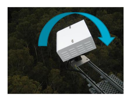
Cameras can move anywhere within +/- 160 degree azimuth +10/-80 degree elevation range.
