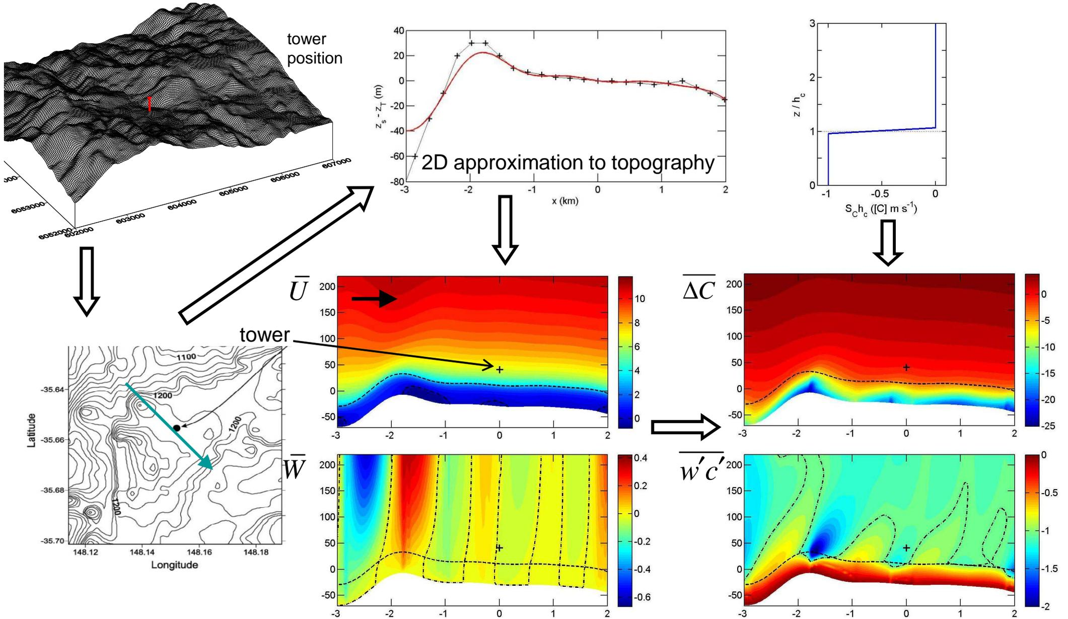
Local perturbations to measured flux due to local and remote topographic features
