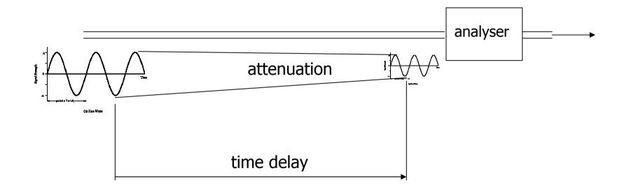
Tubing acts like a low-pass filter by mixing the air Higher frequencies strongly attenuated – depends on:
