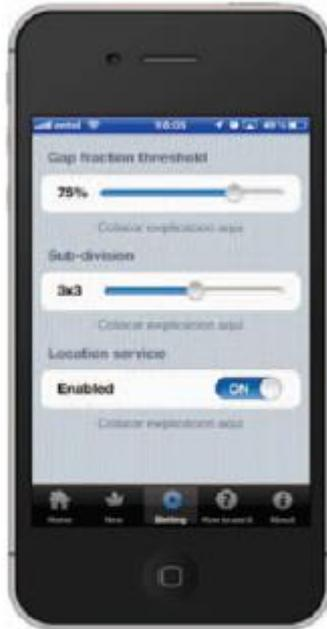
Figure 3. Settings menu showing options for the gap fraction threshold, image sub-division options and to enable/disable the location services from the device.
