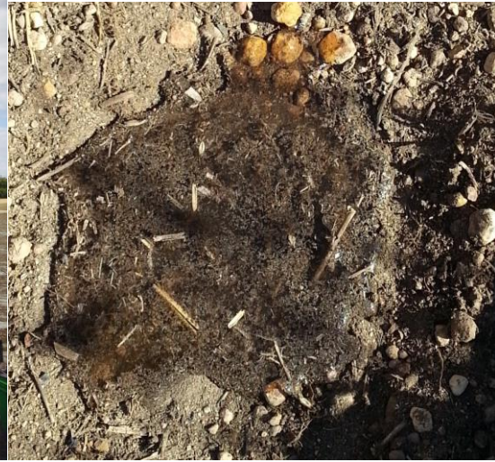
Left: Monitoring of thermal properties on a site effected by water repellency. Right: Severe water repellent soil limiting infiltration of water.
