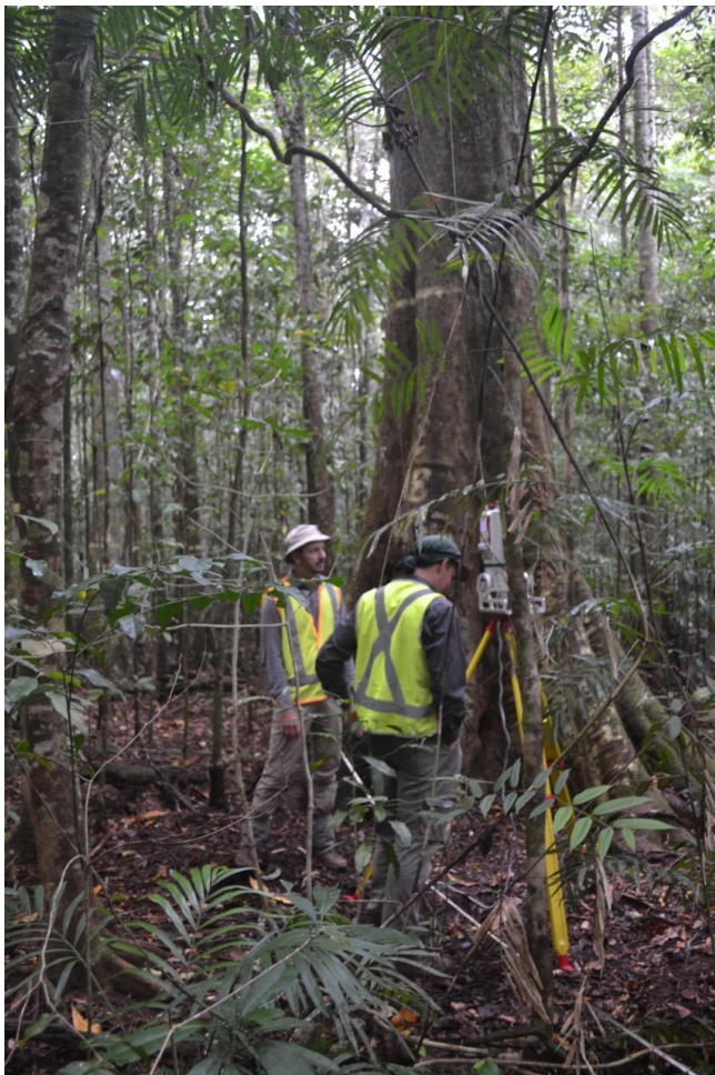
Stuart Phinn and Peter Scarth carrying out Terrestrial Laser Scanning at Robson Creek.
